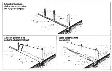
Construction of a silt fence. Source: OMNR (1990).
