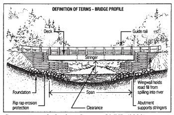
Components of a bridge. Source: OMNR (1990).
