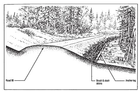
Brush barrier at toe of fill. Source: OMNR (1990).
