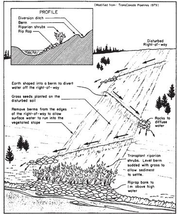
*Erosion control on sloped approaches to streams. Source: British Columbia Ministry of Environment (1986).*
