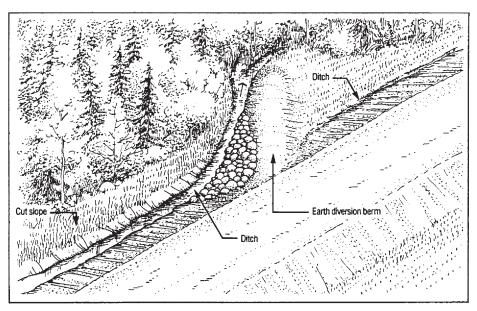
*Forest floor filter - flow directed off right-of-way using a diversion berm. Source: OMNR (1990).*
