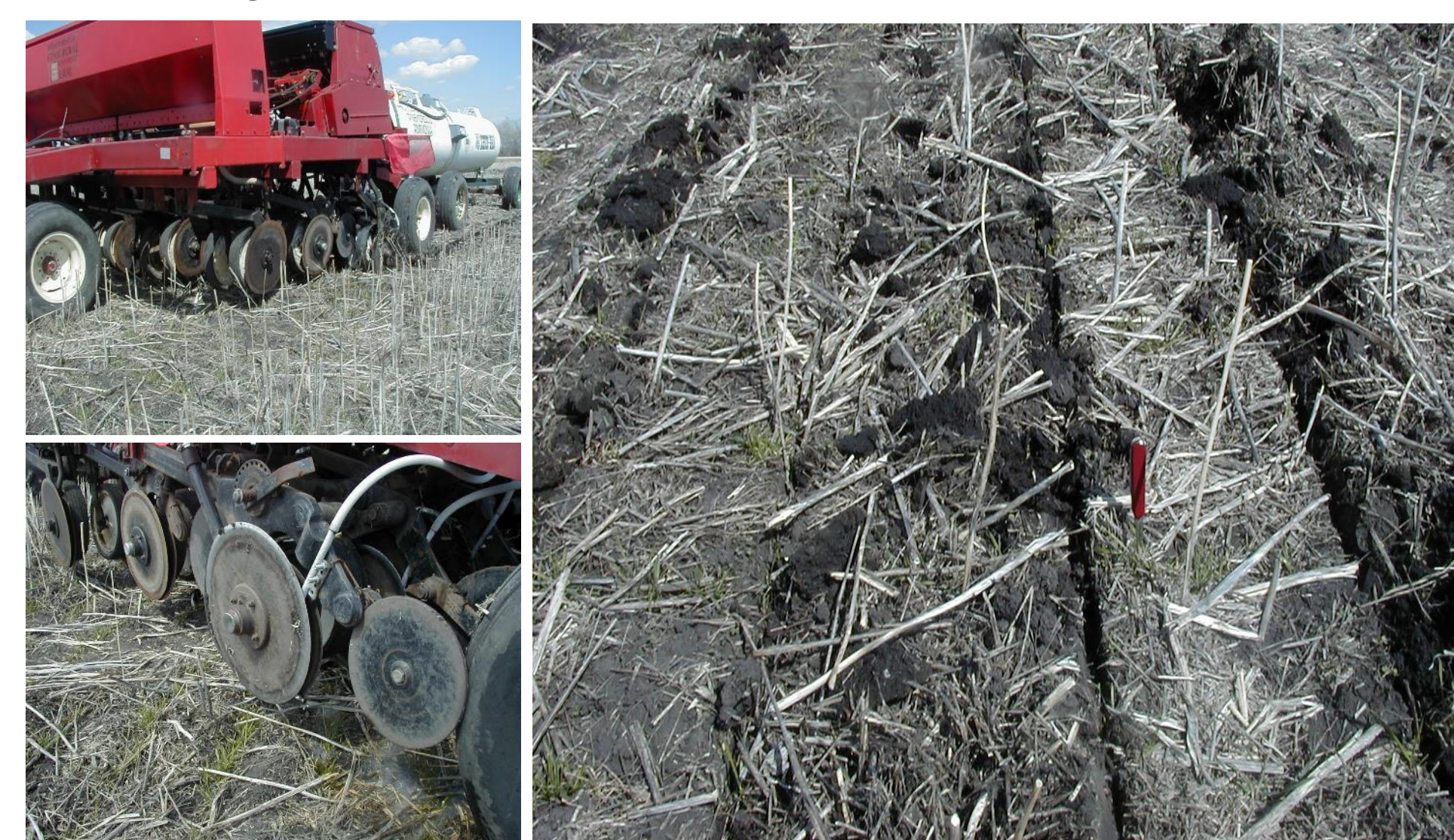
Figure 5. NH_3 placement with Ponik disc opener in spring 2001
