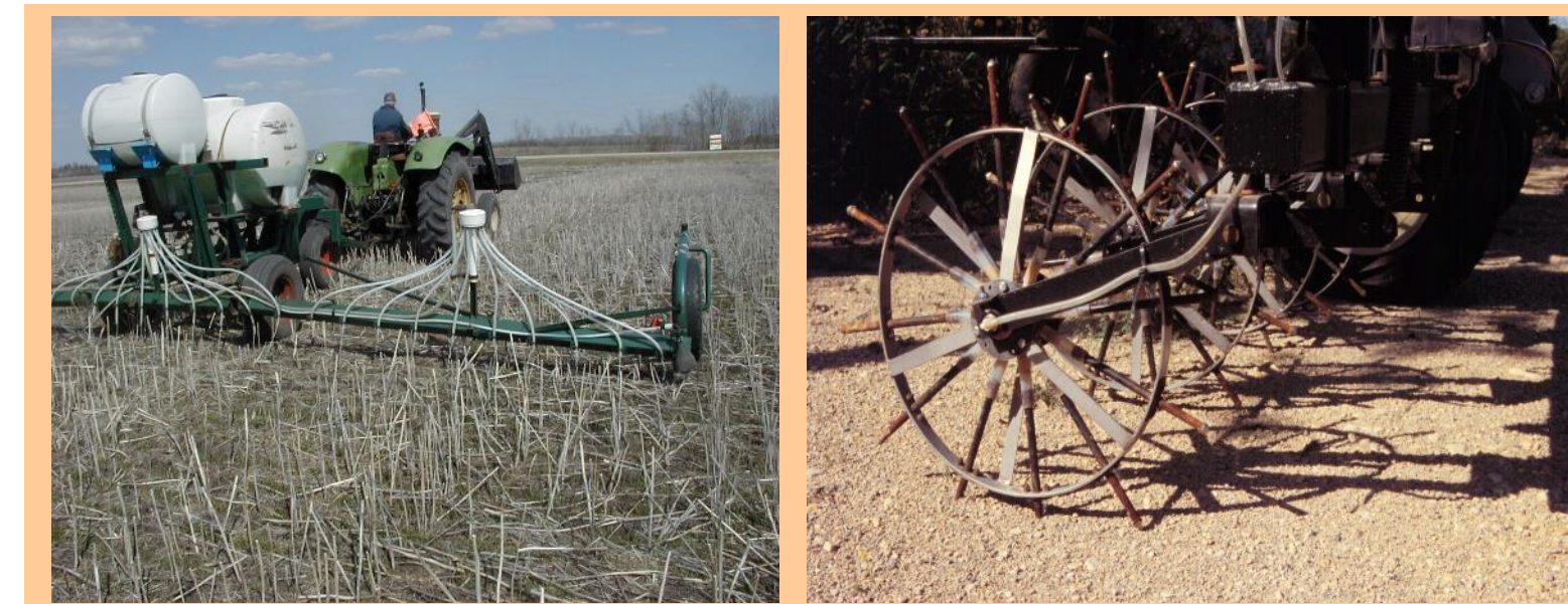
Figure 1. Dribble banded UAN on 12" centres (left) and spoke wheel applicator (right).
